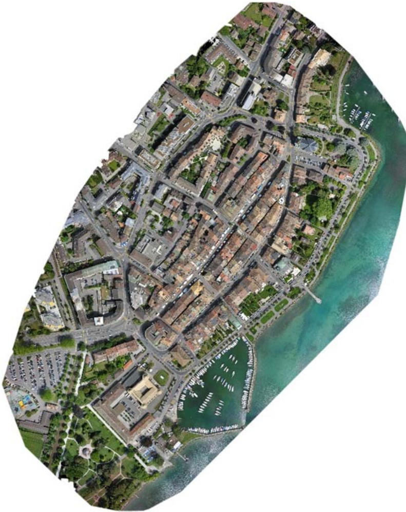
FIGURE 6.1 High-res orthophoto from UAV survey. Courtesy of Pix4D SA.
