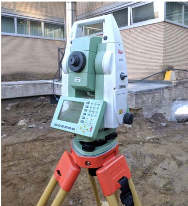
FIGURE 6.5 Robotic total station (photo by the author).
