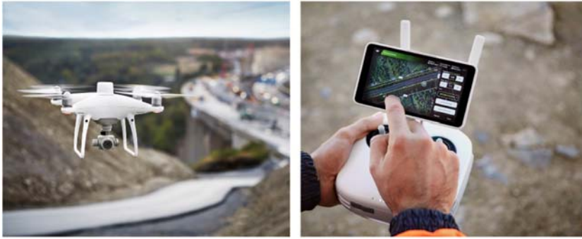
FIGURE 9.14 DJI Phantom IV RTK and remote controller. Courtesy of DJI.
