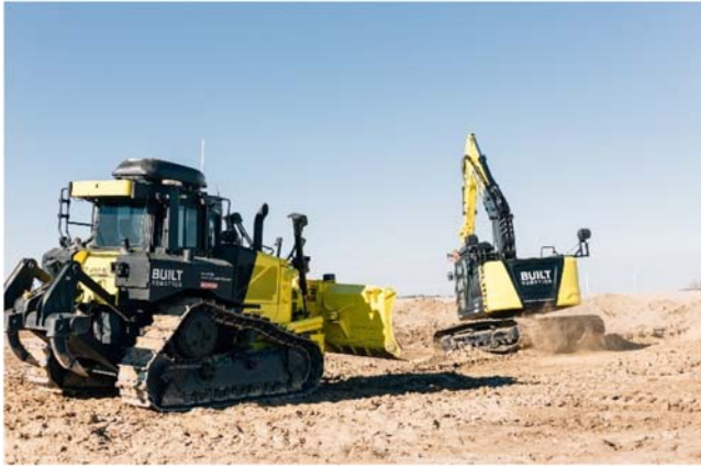
FIGURE 3.10 Autonomous dozer and excavator vehicles. Courtesy of Built Robotics.
