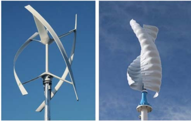
FIGURE 12.21 Darrieus (left) and Savonius (right) wind turbines. Photos by the author.
