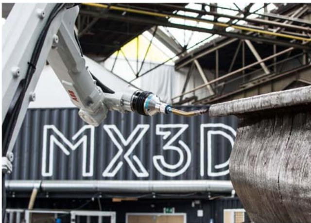
FIGURE 8.27 WAAM DED printing of metal wires. Courtesy of MX3D, photo by Oliver de Gruijter.
