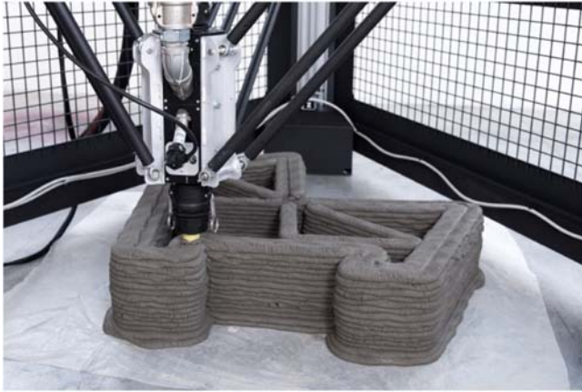
FIGURE 8.34 Delta cement printer. Courtesy of WASP.
