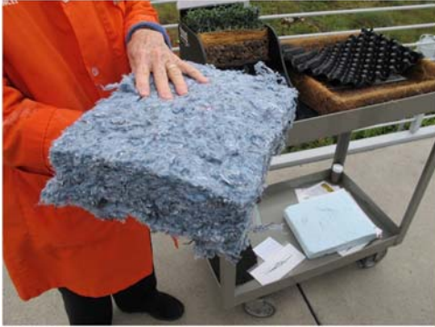
FIGURE 7.4 Recycled jeans insulation. Photo by the author.
