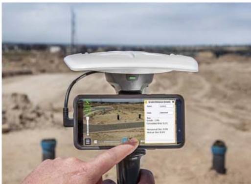
FIGURE 9.24 Trimble SiteVision AR system. Courtesy of Trimble.
