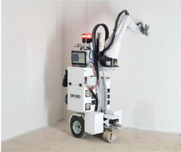
FIGURE 8.9 Okibo wall finishing robot. Courtesy of Okibo.
