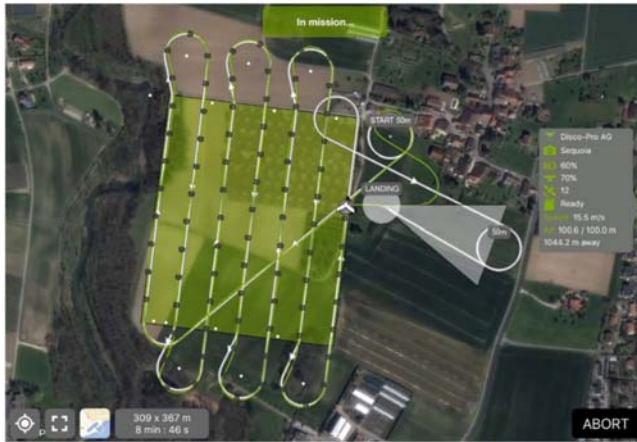
FIGURE 9.11 UAV flight plan and control. Courtesy of Pix4D SA.
