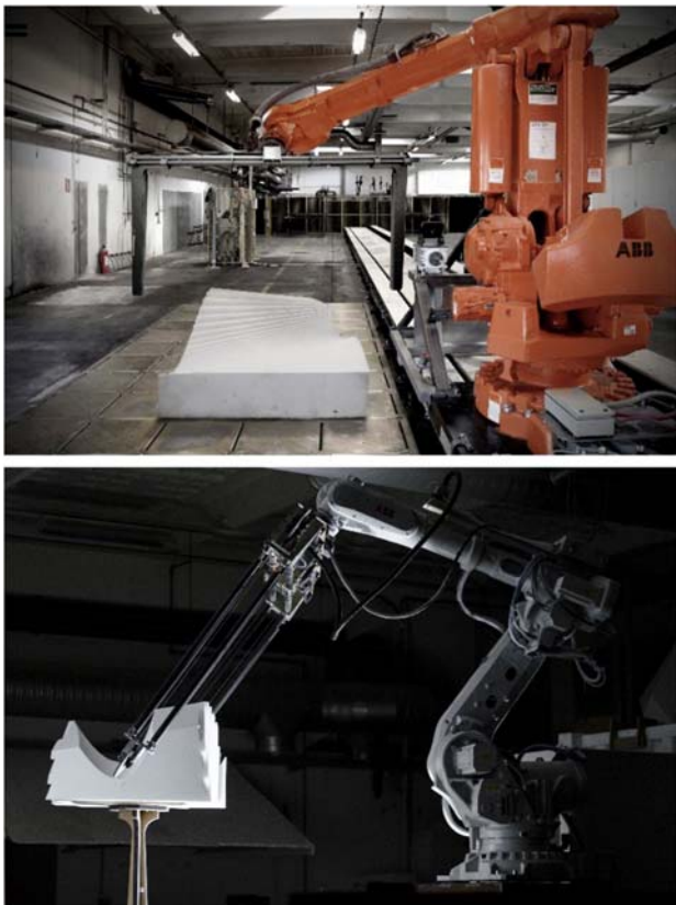
FIGURE 8.6 RHWC (top) and RAWC (bottom) formwork production. Courtesy of ODICO.
