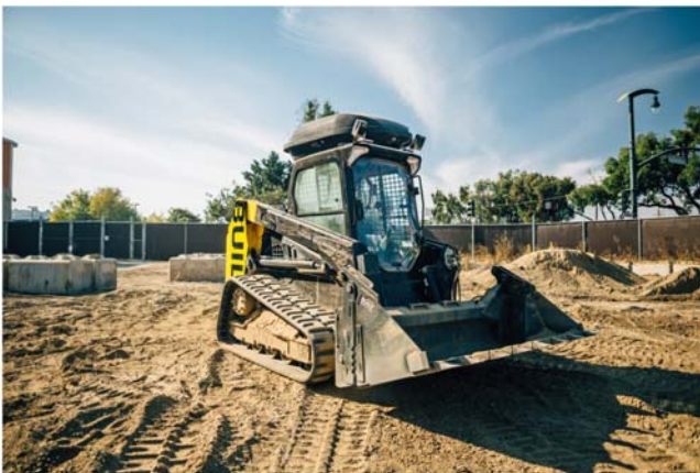
FIGURE 8.20 Built Robotics autonomous CLT. Courtesy of Build Robotics.
