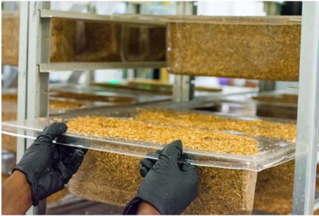
FIGURE 7.7 Mycelium brick preparation. Courtesy of Ecovative.
