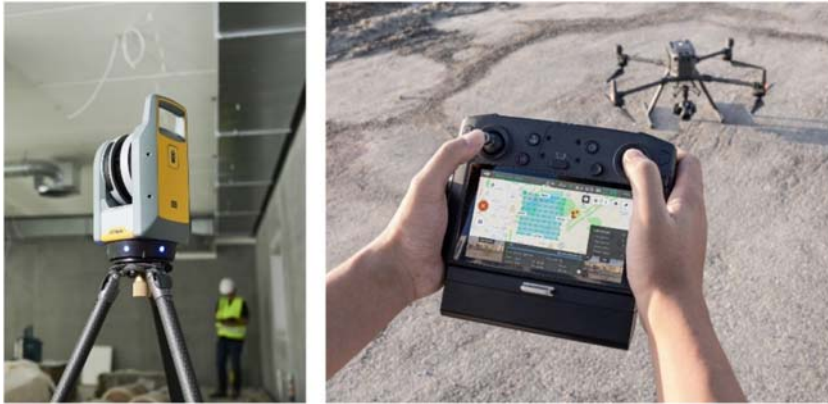
FIGURE 3.4 New LiDAR (left) and drone (right) data acquisition systems. Courtesy of Trimble and DJI.
