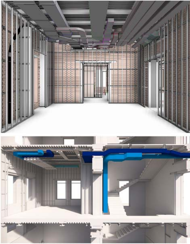
FIGURE 4.2 MEP design with BIM. Courtesy of BIMon.
