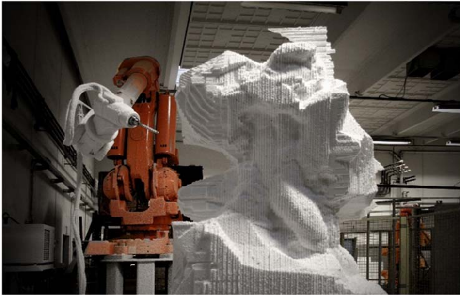
FIGURE 6.41 Multiaxis robotic milling. Courtesy of ODICO.
