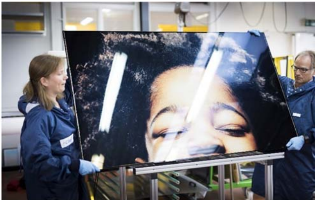
FIGURE 7.40 PV module laminated with printed interlayer. Credit: Kaleo Solar.
