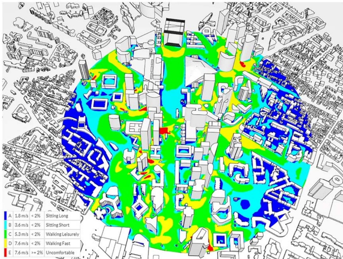
FIGURE 2.9 Local PWC analysis with CFD software.
