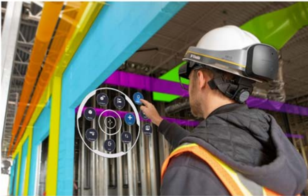
FIGURE 9.26 MR overlay and interaction with BIM model with Microsoft Hololens 2 and Trimble XR10. Courtesy of Trimble.
