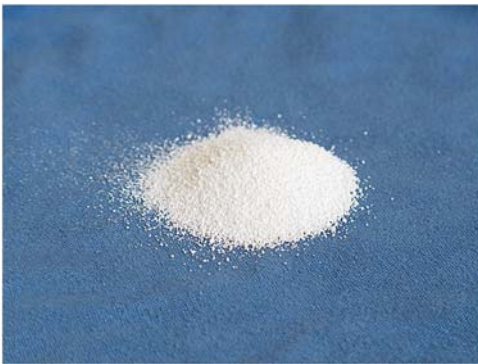
FIGURE 7.23 BASF micronal microencapsulated PCM. Photo by the author.
