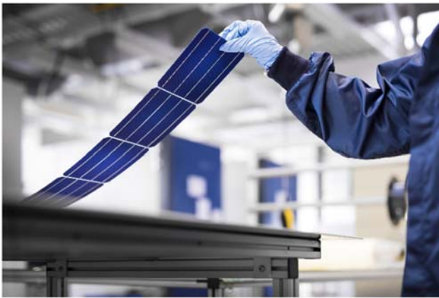
FIGURE 12.17 Crystalline silicon PV cells. Courtesy of Kaleo Solar.
