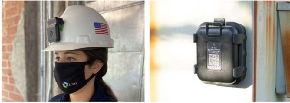
FIGURE 9.22 Spot-r wearable tag (left) and gateway anchor (right). Courtesy of Triax Technologies.
