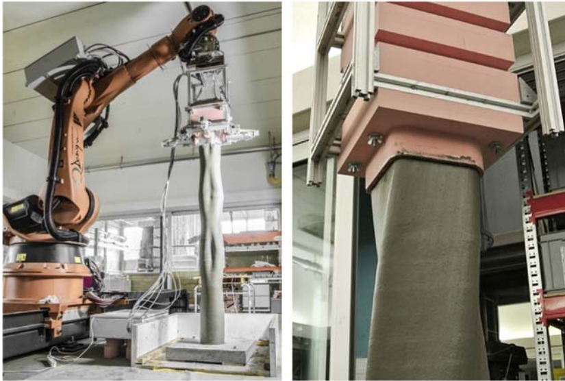
FIGURE 8.3 Smart dynamic casting prefabrication of concrete structures. © Gramazio Kohler Research, ETH Zurich.
