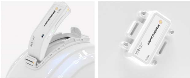
FIGURE 9.21 WorkerSense hardhat sensor and tags. Courtesy of WorkerSense.
