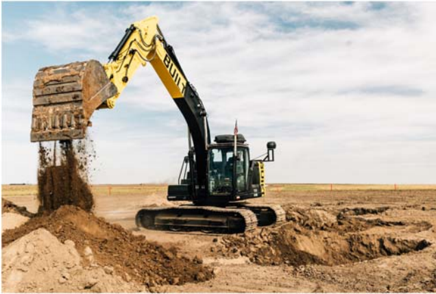
FIGURE 8.18 Built Robotics autonomous excavator. Courtesy of Build Robotics.
