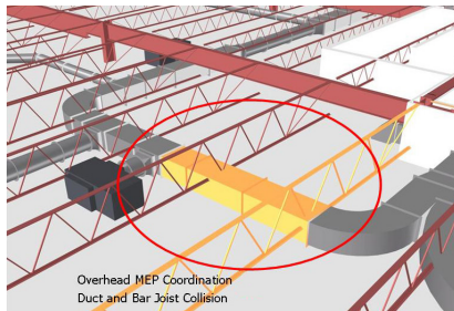
Figure 6 Ductwork conflicts with Bar Joists
