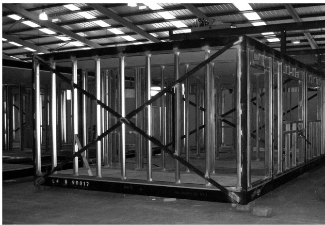
Fig. 1. Light steel module with a perimeter framework (image by R. M. Lawson)
