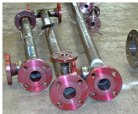
Figure 10.7 Ship piping system, illustrating sectional modularity, (Erikstad 2009)
